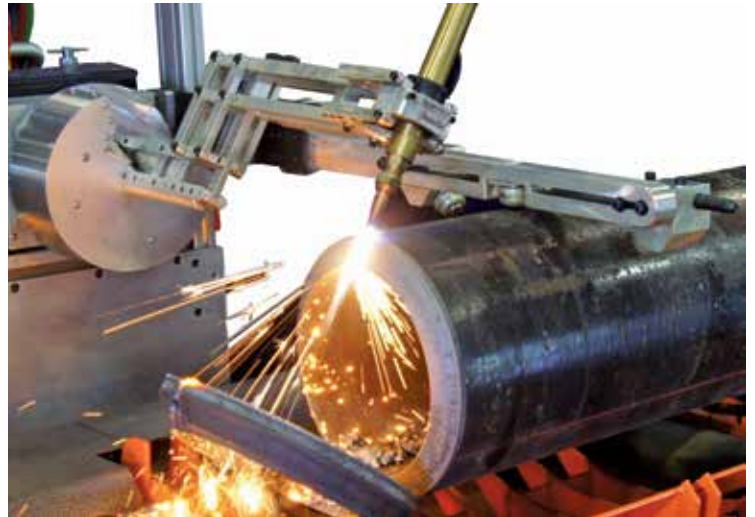
Torch head of a pipe profile cutting machine
