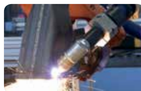
Fasenschneiden Bevel cutting
